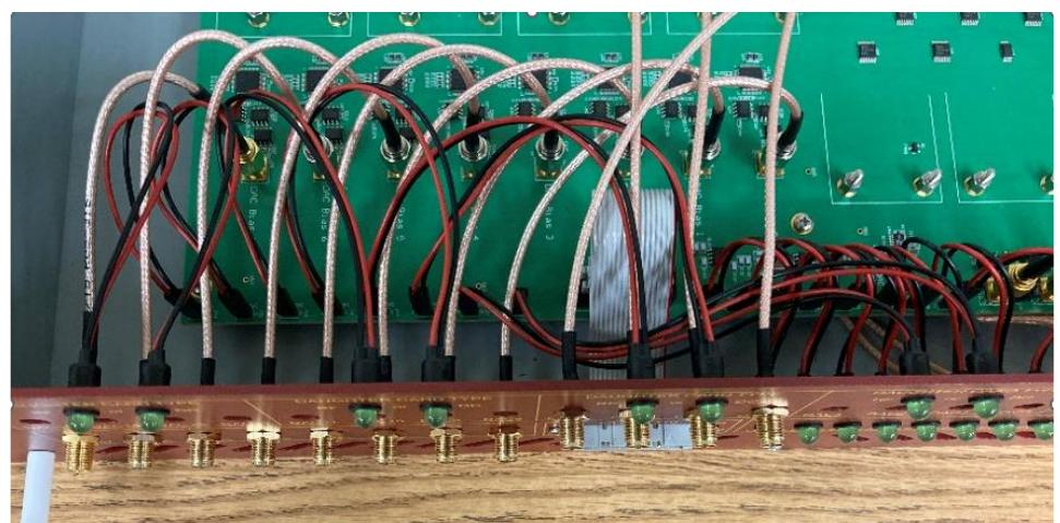
18. Insert eight 3" LEDs (#6) in enclosure front panel holes labeled "RF" and "DC" above the "ADC" SMAs. Connect other end of the eight 3" LEDs to the eight 2-pin headers labeled "ADCxx\_RF" and "ADCxx\_DC" on the RF216 Main board.
