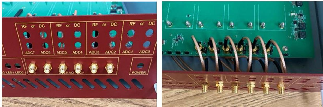
13. Install eight 3" LEDs (#6) in LED 0-7 holes on enclosure front panel. Connect opposite end of those LEDs to 2-pin headers labeled "LED0" – "LED7" on the RF216 Main board. Notice that the headers have one pin labeled "B" (Black) and one pin labeled "R" (Red). Match the wire color of the LED accordingly.
