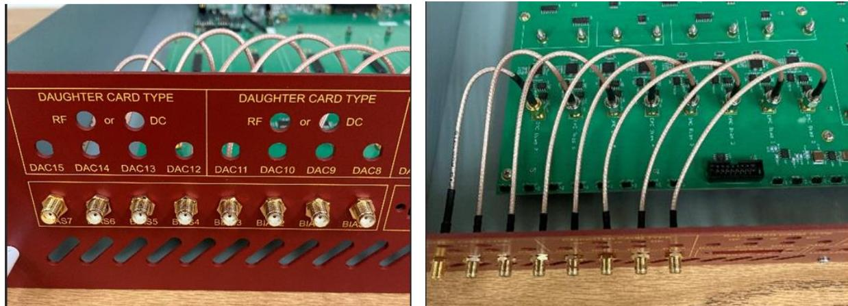
12. Install six 7" SMA cables (#5) in the "USER I/O" 0-5 labeled front panel holes. Use the SMA torque wrench to install opposite end of "USER I/O" SMA cables on "USER I/O" SMA connectors on RF216 Main board.
