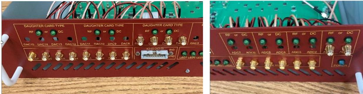
17. Insert eight 6" LEDs (#3) in enclosure front panel holes labeled "RF" and "DC" above the "DAC" SMAs. Connect other end of the eight 6" LEDs to the eight 2-pin headers labeled "DACxx\_RF" and "DACxx\_DC" on the RF216 Main board. The "xx" value of the 2-pin header should match the value of the associated DAC SMA cables. Notice that the 2-pin header has one pin labeled "B" (Black) and one pin labeled "R" (Red). Match the wire color of the LED accordingly.
