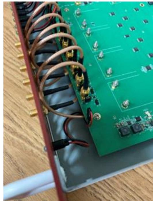
16. Insert as many 15" SMA cables as necessary for your "OUT" and "IN" daughter board configuration into enclosure front panel holes labeled "DACx" and/or "ADCx". "DAC" (Or "OUT" daughter boards) use 4 SMA cables each, and "ADC" (Or "IN" daughter boards) use 2 SMA cables each. Note that daughterboard cables ship with the daughterboards.
