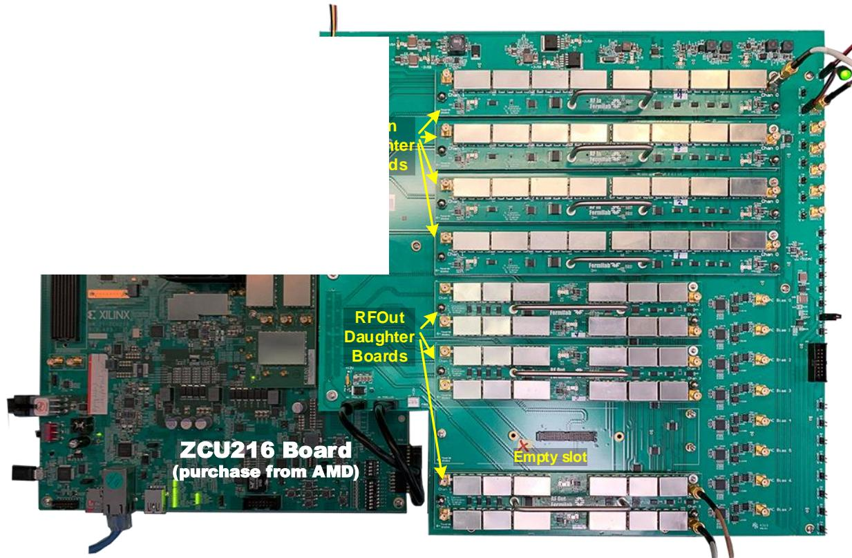
The RF Main board is mounted directly to the ZCU216 board and installed in the QICK case.
